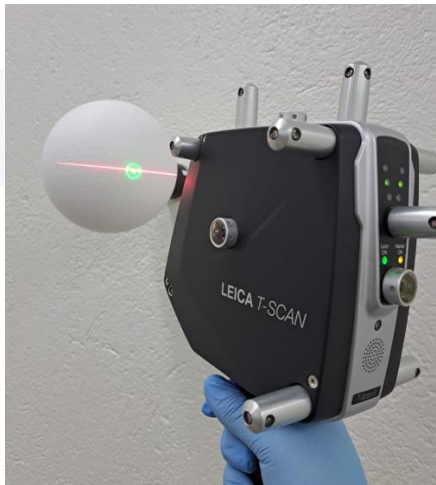
Leica Laser Tracker AT960 + T-Scan
