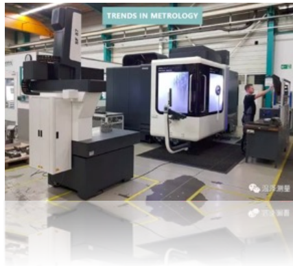
Response to processing centre „closed loop“
