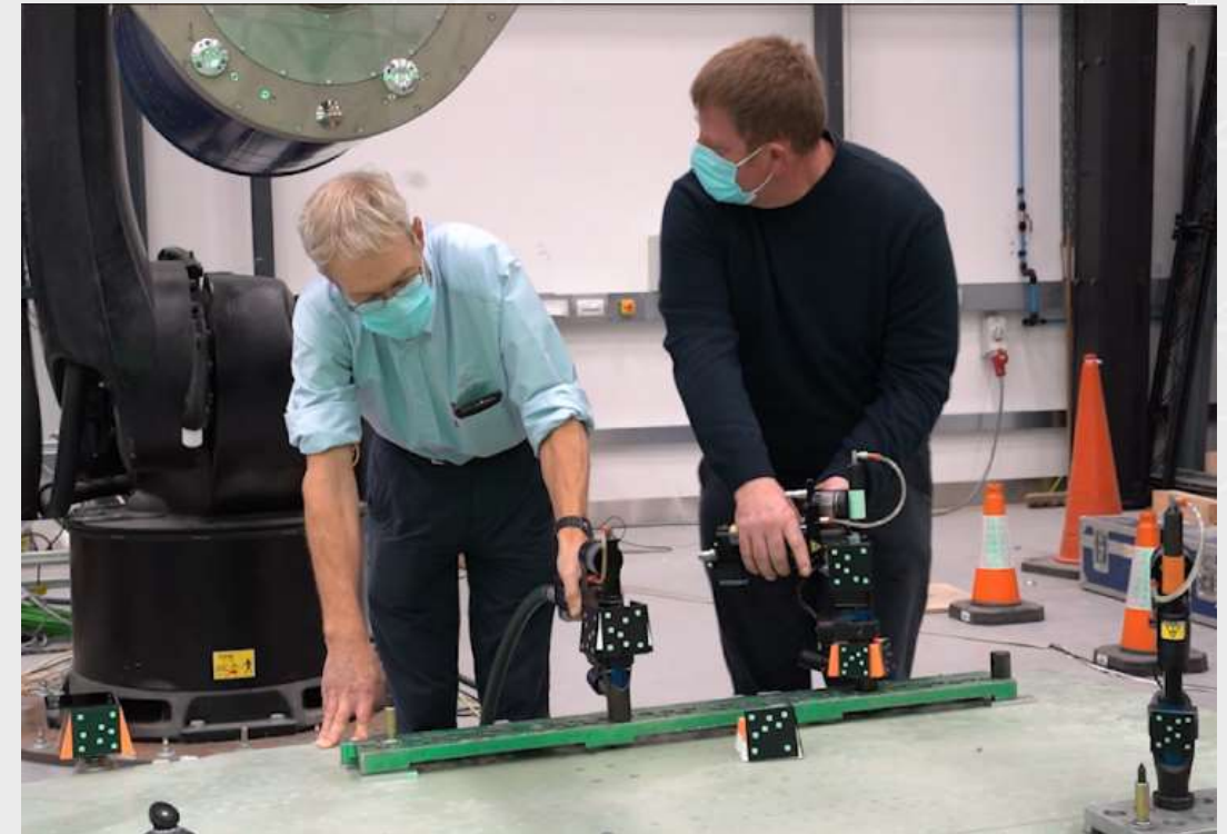
Lab demonstration of low-cost photogrammetry system tracking multiple drilling units at 10Hz
