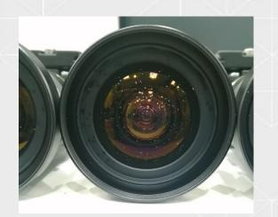
Factory environment led to oil spot contamination of lens surfaces, leading to image distortion. Work is being done to mitigate this. Large-scale CMM Laboratory conditions
