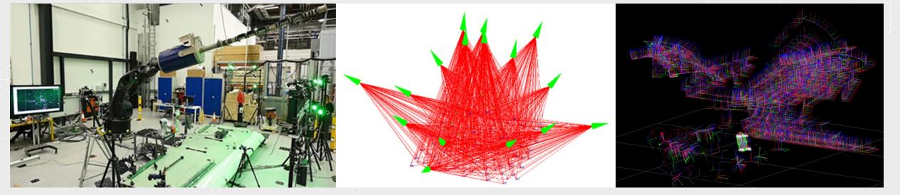
In the low-cost photogrammetry space this project has demonstrated 6DoF solutions scalable in volume, complexity, and number of tracked objects, tracking 50+ 6DoF solutions in parallel within a common spatial and temporal reference system at different frequencies and accuracies. This work investigates the high speed measurement capabilities of this approach.
