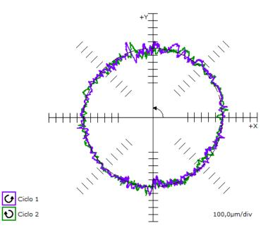
Positioning tolerance: 370,6 microns Better radius: 299,954 mms Circularity: 329,7 microns
