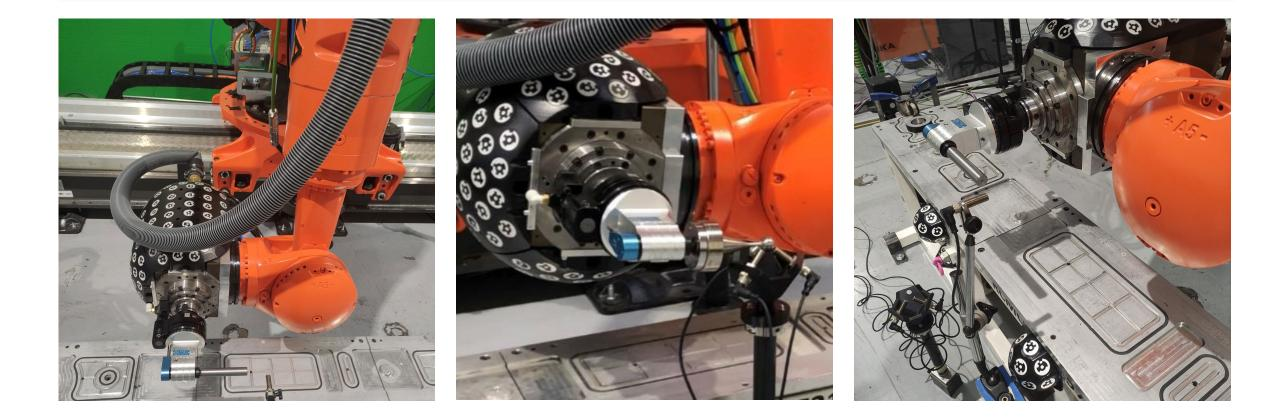
Position measurement of the robot moving along the Y-axis, without and with multi-camera system.
