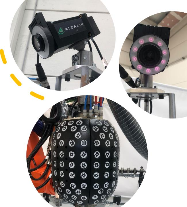
• Calibration of angled tool holders with vision and inductive sensors.
