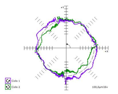
Positioning tolerance: 1735,7 microns Better radius: 300,273 mms Circularity: 557,5 microns 300 mm radius, with multi-camera
