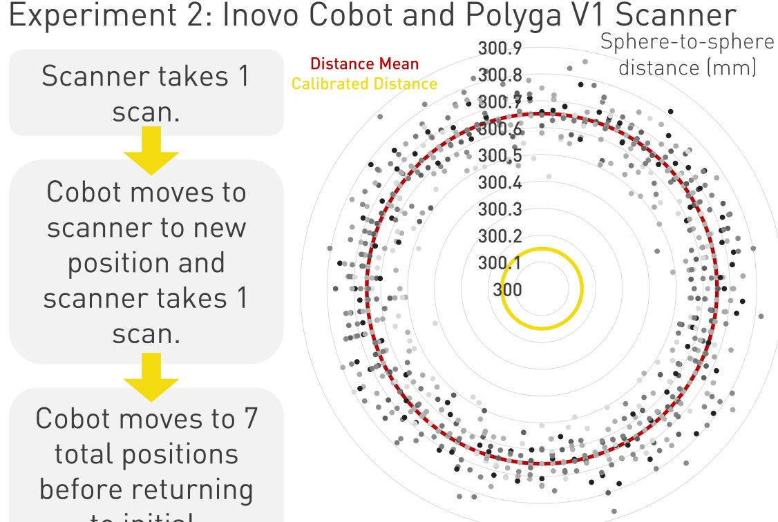
300.652 mm Sphere-to-Sphere Distance Mean 0.503 mm Sphere Spacing Error
