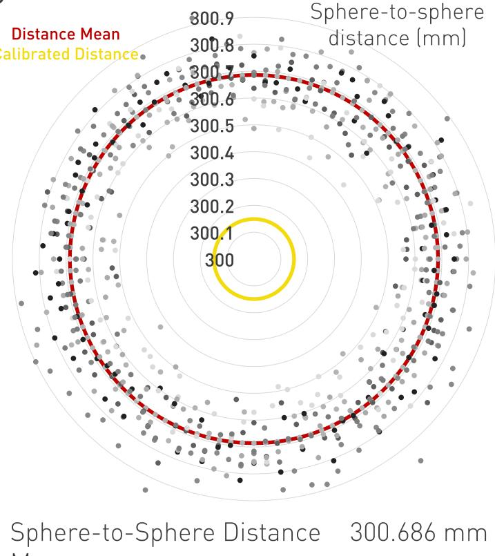
Mean 0.537 mm Sphere Spacing Error
