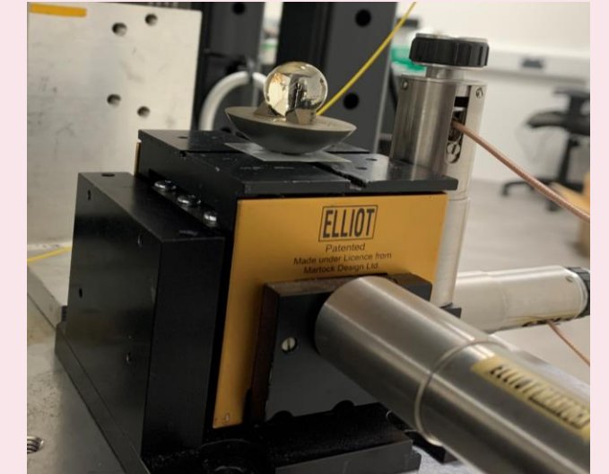
Signal generated by the signal generator stimulate the target movement by changing the OPD of the retro reflector using Elliot piezo vibrator.
